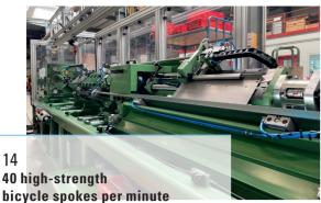
The third generation of Amba's All-in-One reducing machines further improves the straightness of single- and double-butted spokes - as used in electric and cargo bikes, for example.
