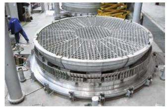
Figure 7: Optimised base design with stationary, highly resistant charging places
