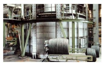
Figure 1. Conti Rotary Table Furnace for solution annealing
