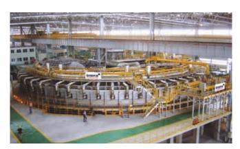
Figure 2. Conti Rotary Hearth Furnace
