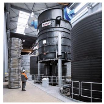
Figure 5. Multi-stack Bell-type Annealing Furnace
