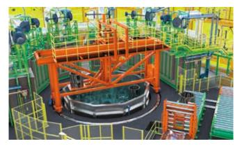
Figure 4. Batch Furnaces incl. quench and manipulators
