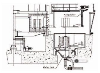
▲ Figure 3. Plant structure of a Conti Rotary Table Furnace with water tank
