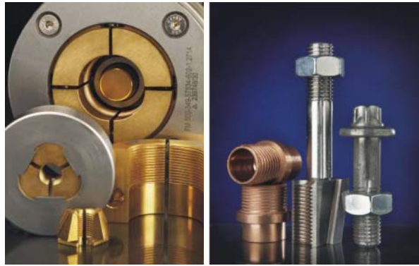
Figure 26: Segmented tools for thread forming (left); Besides massive parts, even hollow parts with external threads can be formed without machining (right) (source: Sieber Forming solutions)
