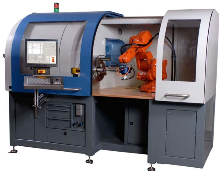
Figure 19: RAP – Robot Assisted Polishing Machine (source: STRECON)
