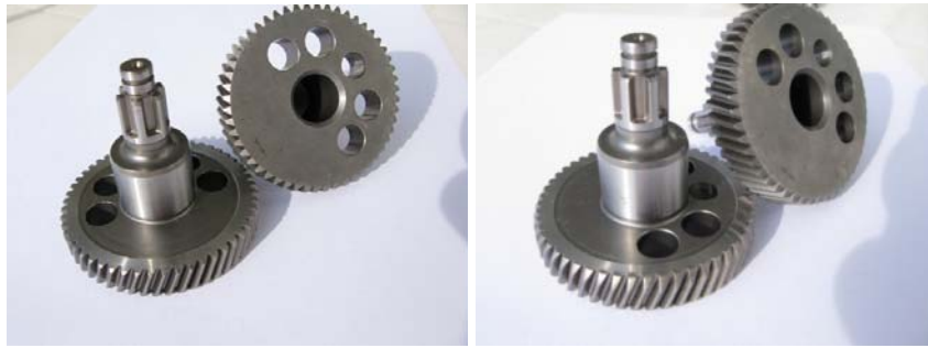
Figure 9: Twin gear drive, straight spline cold forged, helical gear machined (left) and straight spline cold forged, helical gear cold forged in gear quality 9 (right) (source: Wezel)
