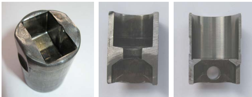
Figure 3: Roller tappet made from 16MnCr5 (left) – hollow forged (middle) and finished with drilling (right) instead of completely drilled, small wall-thicknesses in the corners cause high forming loads (source: Räuchle)
