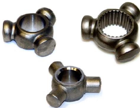
Figure 6: Tripodes – splines and holes in net-shape quality (source: TK Presta)
