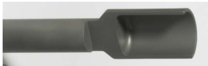
Figure 14: Cold forged hollow shaft made from 28Cr4 manufactured by an automotive company, Germany – Application of a new hardmetal grade from Japan in combination with STRECON stripwound container increases tool life from 24000 to 33000 parts (source: STRECON)
