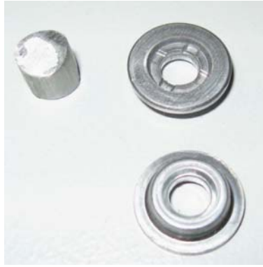
Figure 4: Spacer disk made from aluminum – forged instead of drilled (source: Rächle)
