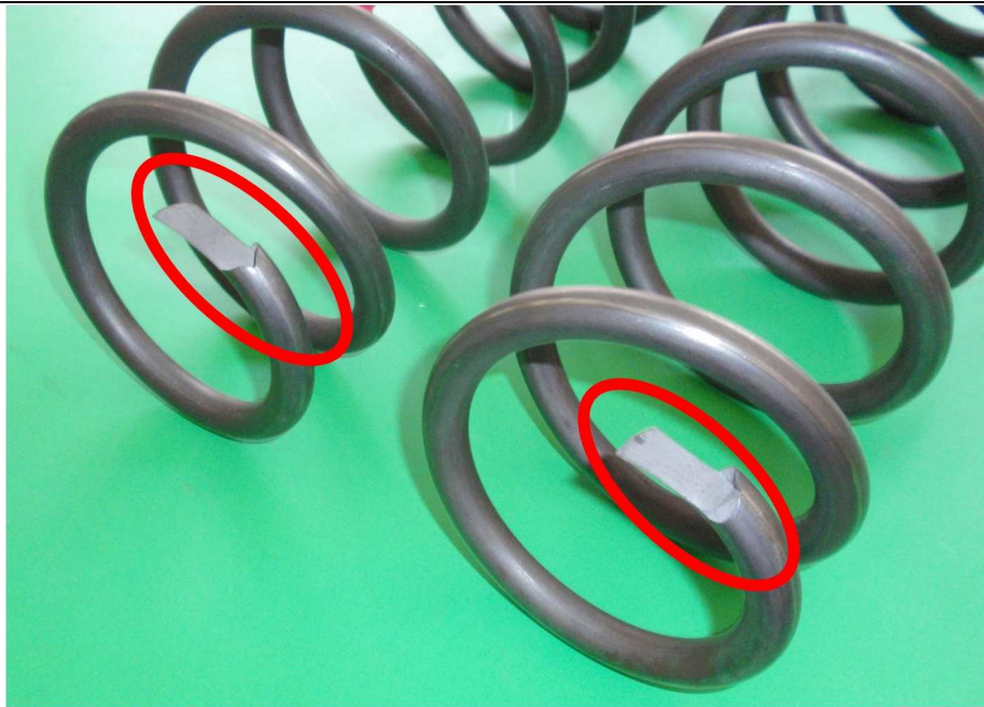
Figure 3. The cracked coiled springs.
