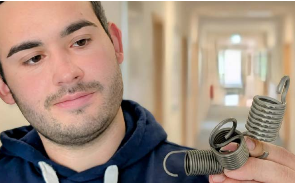
Fig. 1a: Selection of loops investigated in the project (from left to right): half German loop, English loop, and German side loop (C. Otto). © TU Ilmenau
