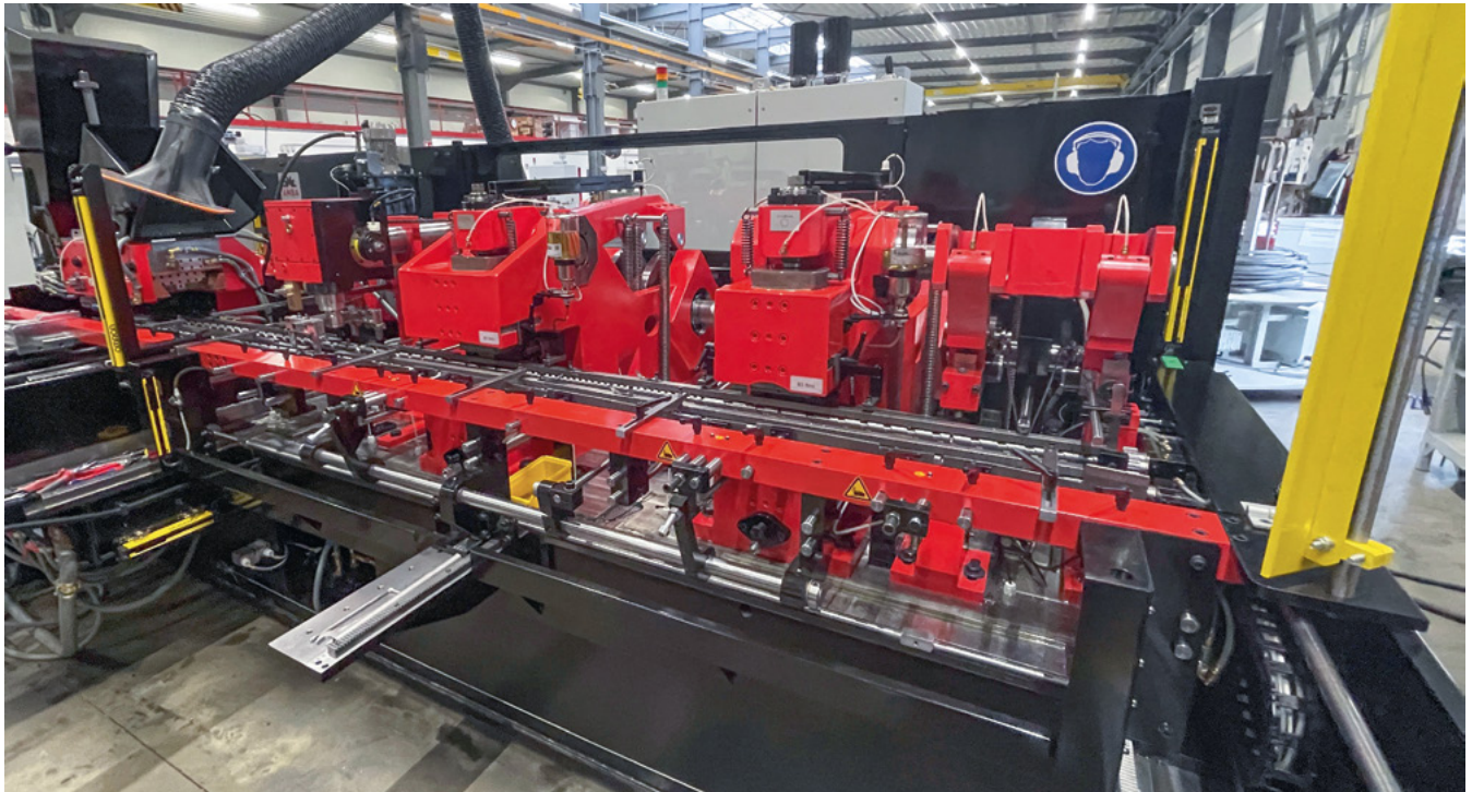
The new "BM 12" is the first screwmaking machine able to produce up to 70 screws per minute from 18-mm-Ø wire. © Aachener Maschinenbau
