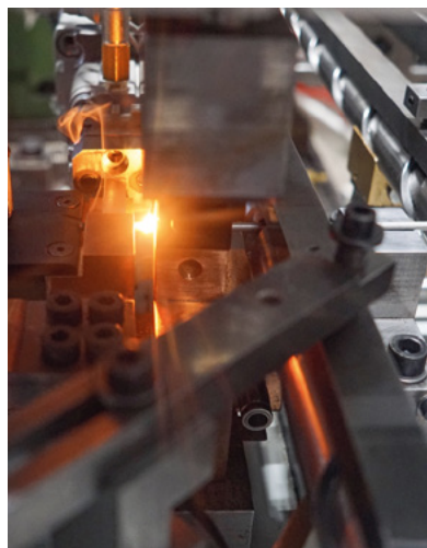
Weld joining of the carbon steel drill point to the stainless steel blank in the new "BM-BiMetal" machine.
